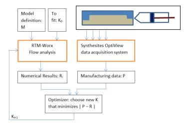
Figure 1: Overview of the model identification procedure.
